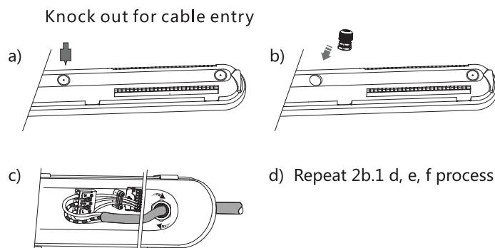
Switch off the power supply before installation
