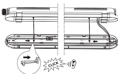
Use only optical sub-assembly that delivered with housing in one box!
